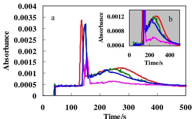
**Figure 4.** (A) Electropherograms of HAs analyzed with tetraborate buffer (pH 9.18) [20 kV, 25°C, detection at 200nm]. (—) AHA; (—) IHA; (—) DHA; (—) BHA. The inset (B) is the close view of the second peak of (A).
