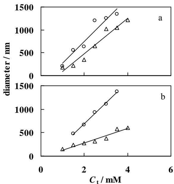
**Figure 7.** Dependence of hydrodynamic diameter of the  $\text{C}_{12}\text{Py}^+$ -AFA and  $\text{C}_{12}\text{Py}^+$ -AHA aggregates on total surfactant concentration at pH 9.18 and at ionic strength ( $\Delta$ ) 0.03M, (o) 0.10M. (a) AFA system, (b) AHA system.
