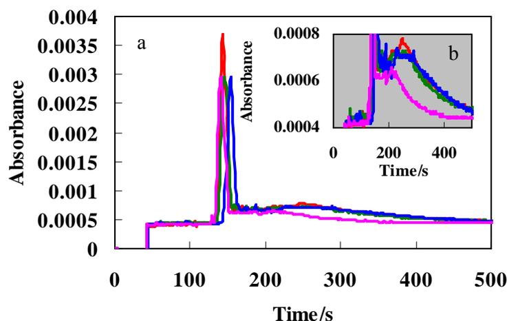
**Figure 7.** (A) Electropherograms of FAs analyzed with tetraborate buffer (pH 9.18) [20 kV, 25°C, detection at 200nm]. (—) AFA; (—) IFA; (—) DFA; (—) BFA. The inset (B) is the close view of the second peak of (A).
