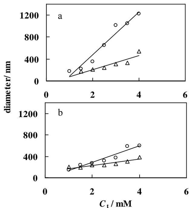
**Figure 6.** Dependence of hydrodynamic diameter of the cationic surfactant-HS aggregates on total surfactant concentration at pH 9.18 and ionic strength  $0.03 \text{ mol dm}^{-3}$  (a) AFA system, (b) AHA system. (o)  $\text{C}_{12}\text{Py}^+$ , ( $\Delta$ )  $\text{DTMA}^+$ .
