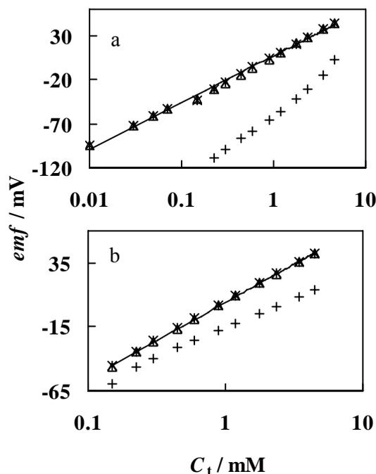
**Figure 1.** Potentiograms of (a) C<sub>12</sub>Py<sup>+</sup>-IHA system and (b) C<sub>12</sub>Py<sup>+</sup>-IFA system. (Δ); (\*) without FA or HA; (+) with FA or HA; pH = 9.18, I = 0.03, T = 25°C.
