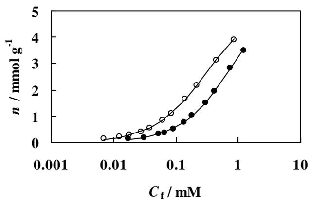
**Figure 5.** Binding isotherms of DTMA<sup>+</sup>-AHA and C<sub>12</sub>Py<sup>+</sup>-AHA system at pH 9.18 ( $I = 0.03 \text{ mol dm}^{-3}$ ).
