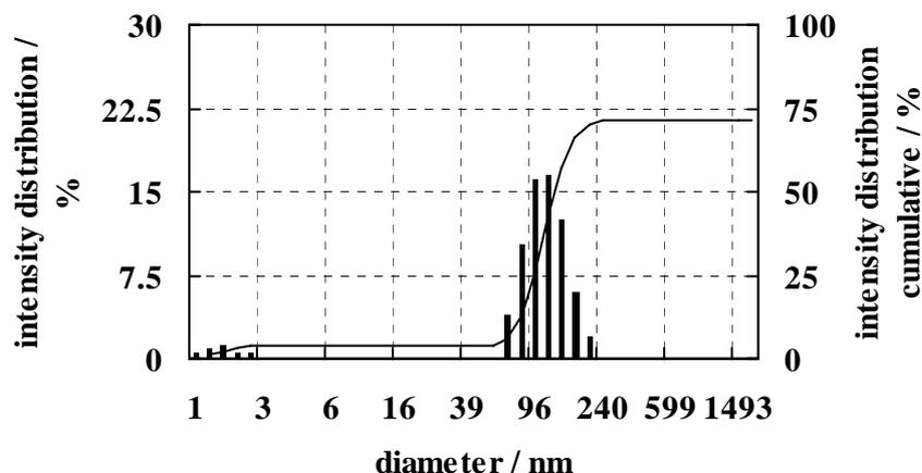
**Figure 2.** Representative histogram of the particle size distribution for  $C_{12}Py^+$ -AHA system ( $3.5 \text{ mmol dm}^{-3} C_{12}Py^+$  and  $AHA 0.05 \text{ g dm}^{-3}$ ) at pH 3.98 and ionic strength 0.10M.
