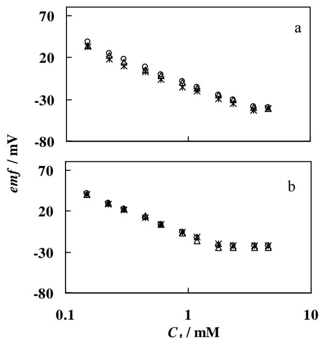
**Figure 1.** Potentiograms of SDS-AHA system (a) at pH 9.18 ( $I = 0.03 \text{ mol dm}^{-3}$ ) and (b) at pH 3.98 ( $I = 0.10 \text{ mol dm}^{-3}$ ).
