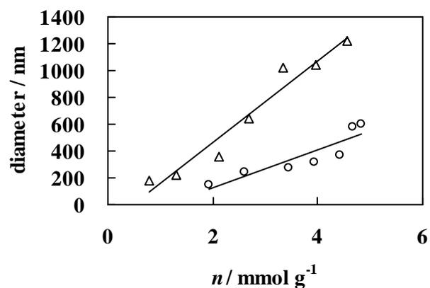
**Fig. 6.** Dependence of hydrodynamic diameter of the  $\text{C}_{12}\text{Py}^+$ -AFA and  $\text{C}_{12}\text{Py}^+$ -AHA aggregates as a function of binding degree: ( $\Delta$ ) AFA system, (o) AHA system.
