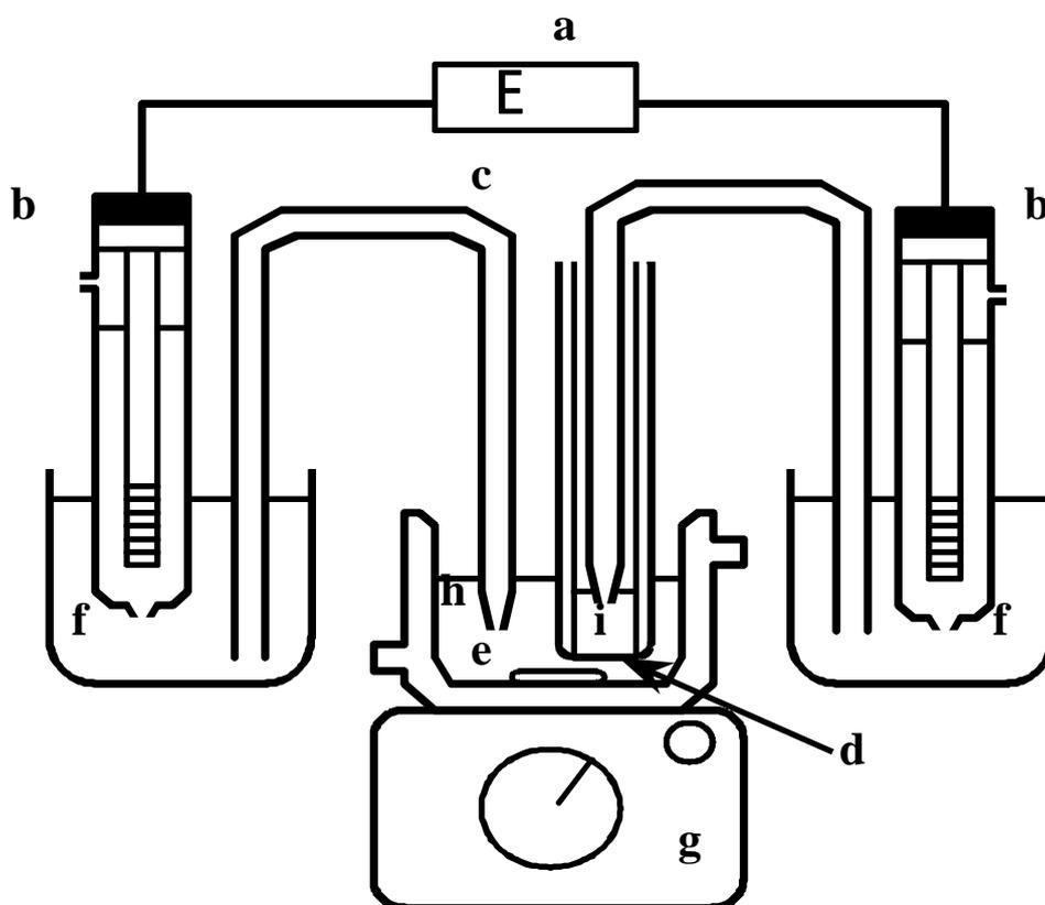
**Figure 5.** The Schematic diagram of surfactant-ion-selective membrane electrode
