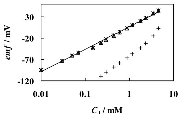
**Figure 6.** Example of potentiometric titration curve determined with cationic surfactant electrode. System: Inogashira Humic acid (IHA) (1 g/ L)-dodecylpyridinium bromide, ( $\Delta$ ); (\*) without IHA; (+) with IHA; pH = 9.18,  $I = 0.03$ ,  $T = 25^\circ\text{C}$ .
